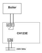
PLEASE NOTE: when CH123E is disconnected, the boiler contact remains in its current position.
